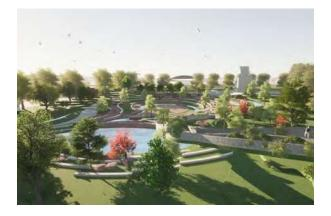
rainwater is purified by layers of wetland plants between the steps by the wetland plants, flows into a circular strip pond in the middle of the wetland, which then converges into an oval-shaped pond.
