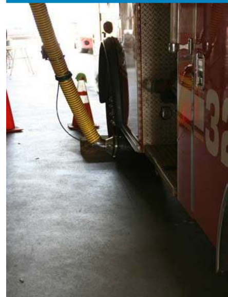
Figure 1.2 — A typical apparatus exhaust system connection.
