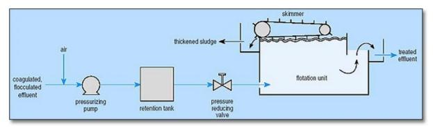
Gas is injected into the water to be treated and particulates and oil droplets suspended in the water are attached to the air bubbles and they both rise to the surface. As a result, foam develops on the surface, which is commonly removed by skimming. The dissolved gas can be air, nitrogen, or another type of inert gas. Dissolved air/gas flotation can also be used to remove volatile organics and oil and grease. Dissolved air flotation units have been widely used for treatment of produced water.
