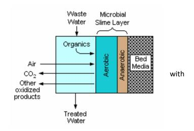
BAF is a well-established technology and has been used for produced water treatment for many years. Because of this technology's ability to remove oil and grease, it has been primarily used for oil-field produced water treatment. Informal versions of BAFs require minimal equipment, can be made by flowing water over rock beds. These types of BAFs have also been used in coal bed methane produced water treatment for iron and suspended solids removal.
