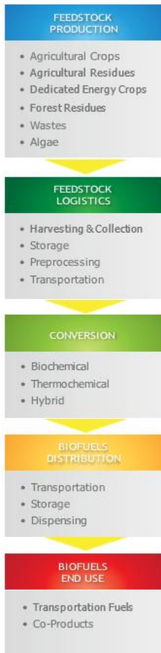
Figure 3. The biofuels supply chain has five major components: (1) feedstock production, (2) feedstock logistics, (3) conversion, (4) distribution, and (5) end use.
