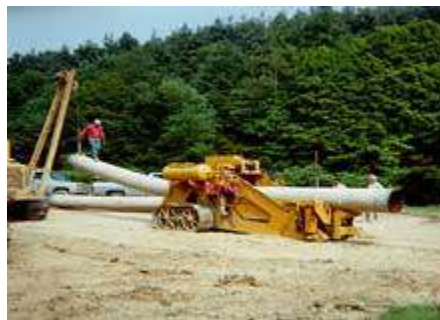
FIGURE 3.3-11 Pipe Bending Machine
