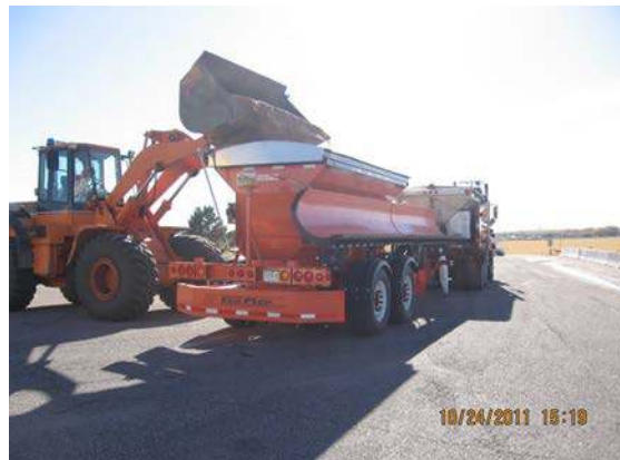
Figure CO-2. Tow plow being loaded with salt.
