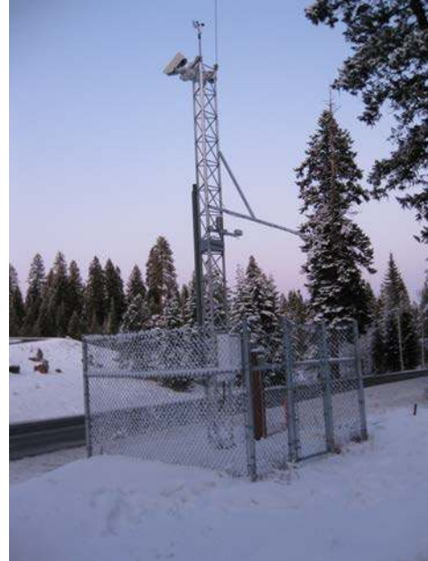
Figure ID-1. RWIS installation at Goose Creek Summit on State Highway 55 in central Idaho.
