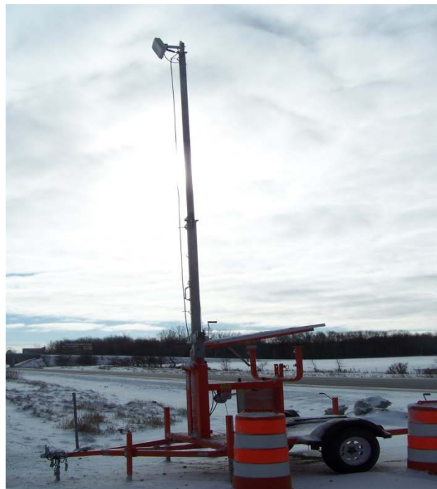
Figure MI-1. Speed sensor apparatus to determine regain time.
