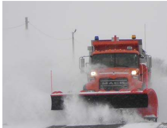
Figure CO-1. Truck with 14 ft. wide front plow.
