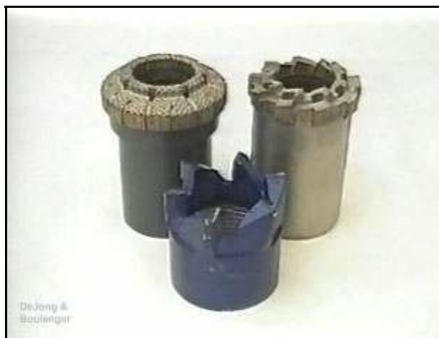
Figure 3-19. Coring Bits. From left to right: Diamond, Carbide, & Sawtooth.
