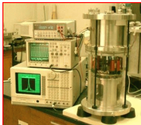
Figure 7-12. Resonant Column Test (RCT) Equipment for Determining G_{\max} and D in Soils.
