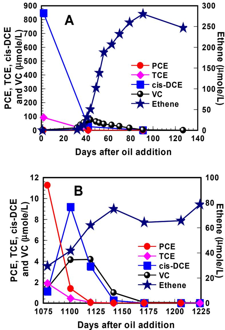
**Figure D.9 Chlorinated Solvent Reductive Dechlorination Over Time.** From one addition of 500 mg/L liquid soybean oil: (a) shortly after microcosm construction; and (b) after repeatedly re-spiking with additional PCE over three years.
