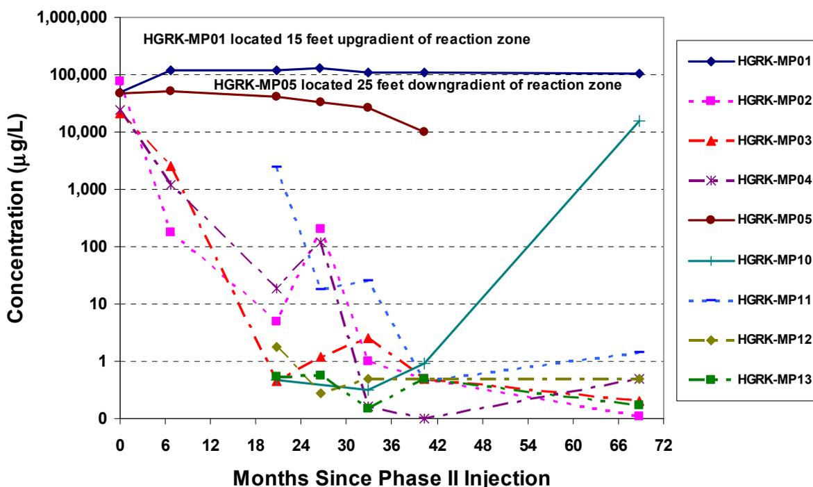
Concentrations of *cis*-1,2-DCE in Phase II monitoring points initially showed variable trends following the Phase II vegetable oil injection. Concentrations of *cis*-1,2-DCE increased at three locations and decreased at four locations in February/March 2001. An increase in *cis*-1,2-DCE is inferred to result from reductive dechlorination of TCE, while a decrease in *cis*-1,2-DCE is inferred to result from subsequent degradation of *cis*-1,2-DCE to VC.
