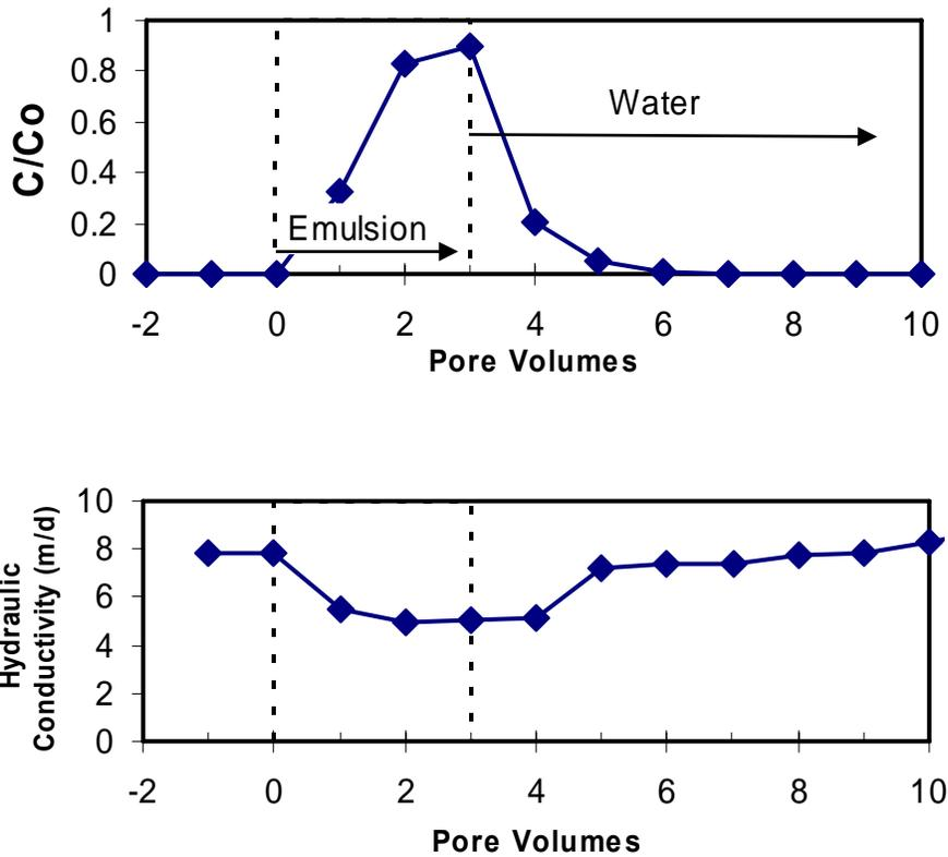
**Figure D.12** Variation in Emulsion Concentration ( $C/C_o$ ) in Column Effluent and Effective Hydraulic Conductivity during Injection in Field Sand with 3 Pore Volumes of Fine Emulsion followed by Plain Water (from Coulibaly and Borden, 2004)
