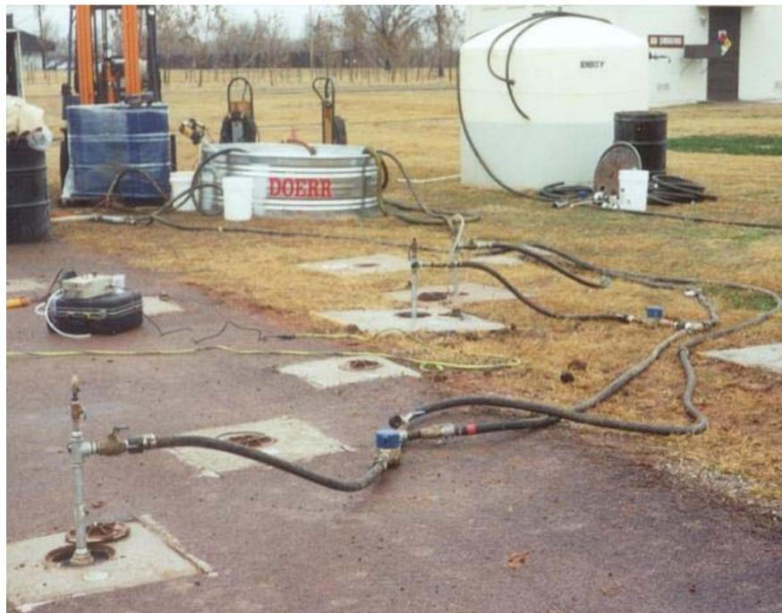
**Figure 1.8** Typical Oil Emulsion Injection System Layout
