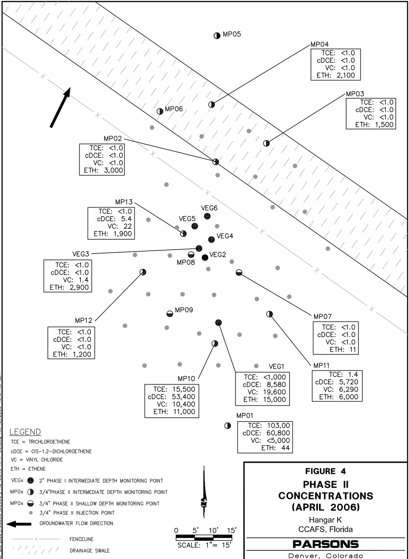
HGRK-MP10. The concentration of TCE rebounded at this location to 15,500  $\mu\text{g/L}$  in April 2006, compared to less than 1.0  $\mu\text{g/L}$  in December 2003. This monitoring location is on the upgradient side of the treatment zone, and the rebound suggests that the treatment zone may no longer be able to degrade elevated concentrations of TCE migrating from an upgradient source.
