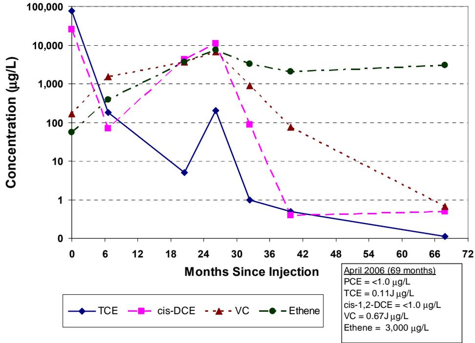
**Figure 7. Concentrations of Chlorinated Ethenes at Downgradient Location HGRK-MP04**
