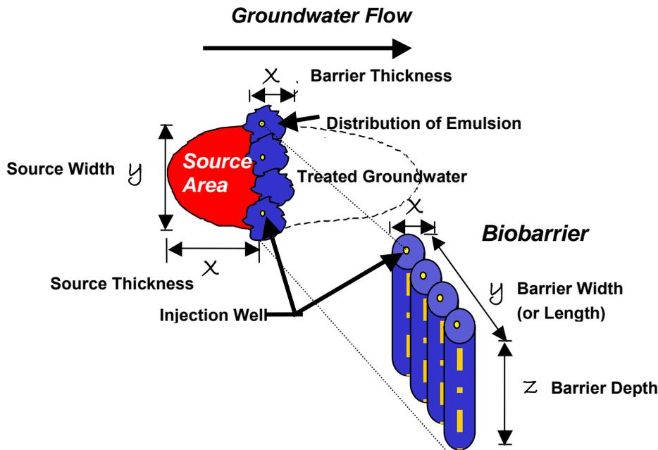
**Figure 4.2 Dimensions Used in Calculating a Treatment Zone**
