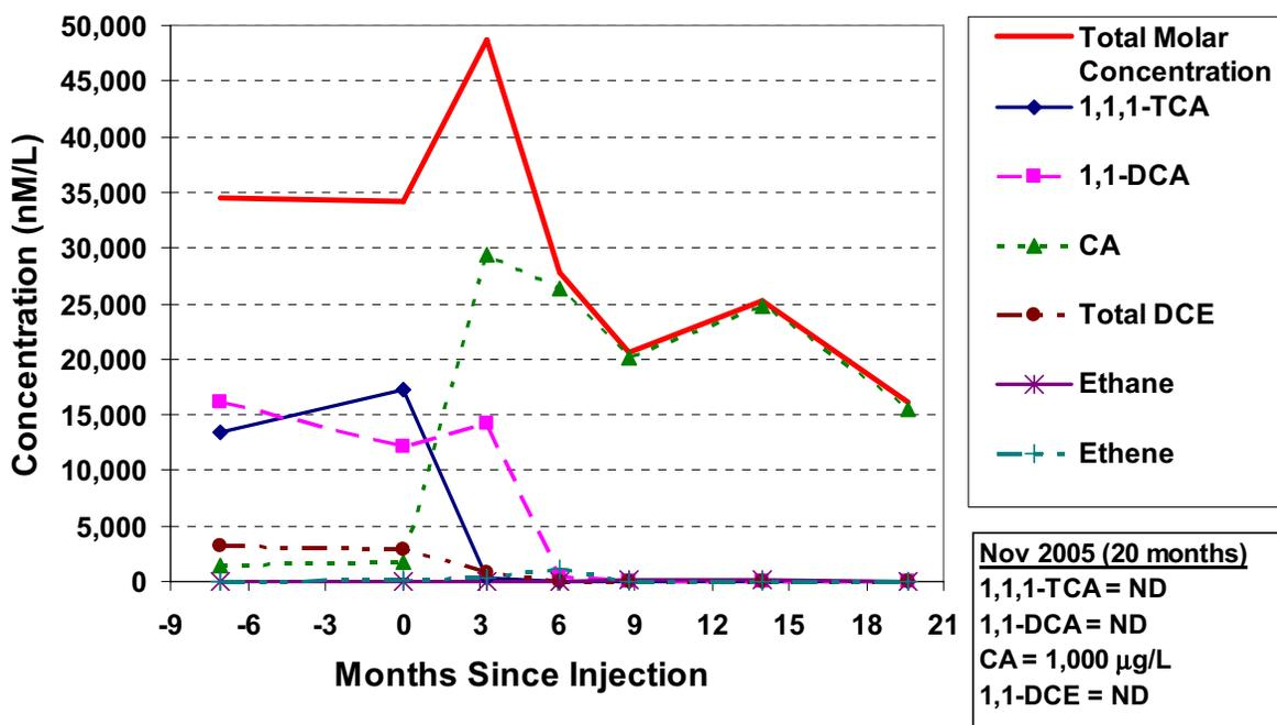
Figure 6 is a plot of the total molar concentration for wells located along the axis of the plume. Each plotted line represents a subsequent sampling event, and it is evident that after the first post-injection sampling event the total molar concentrations along the entire plume axis have been reduced.
