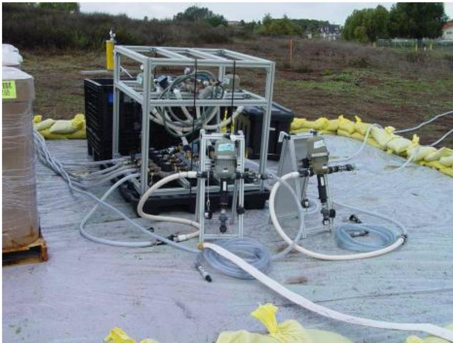
**Figure 5.11 Proportional Feed System for a 10-Line Injection System** (Photo courtesy of Remediation and Natural Attenuation Services, Inc.)
