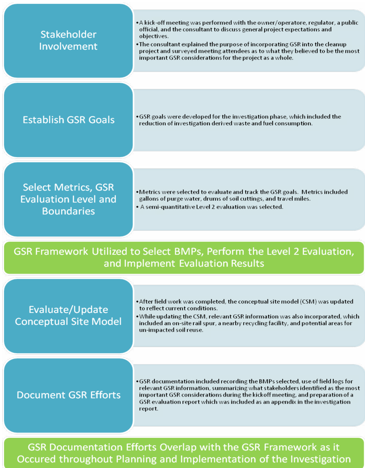
Figure 2-2. Hypothetical example of GSR planning process during the investigation phase of a brownfield project.
