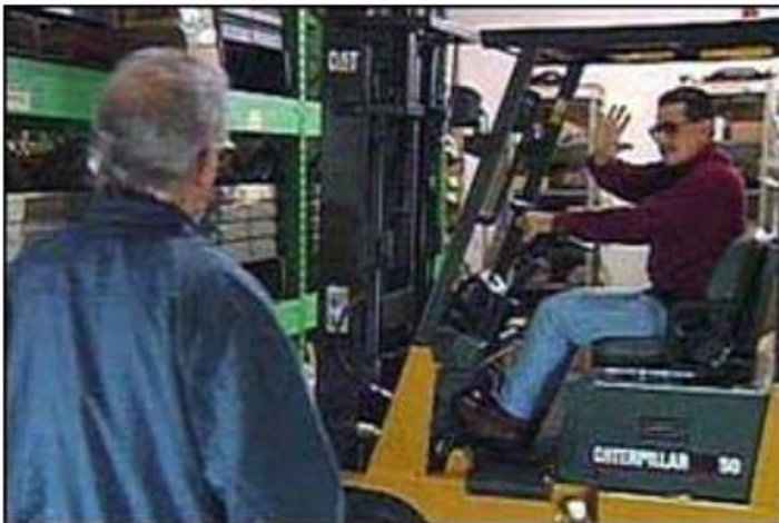
Figure 7. Operator signaling to coworker to stand back.
