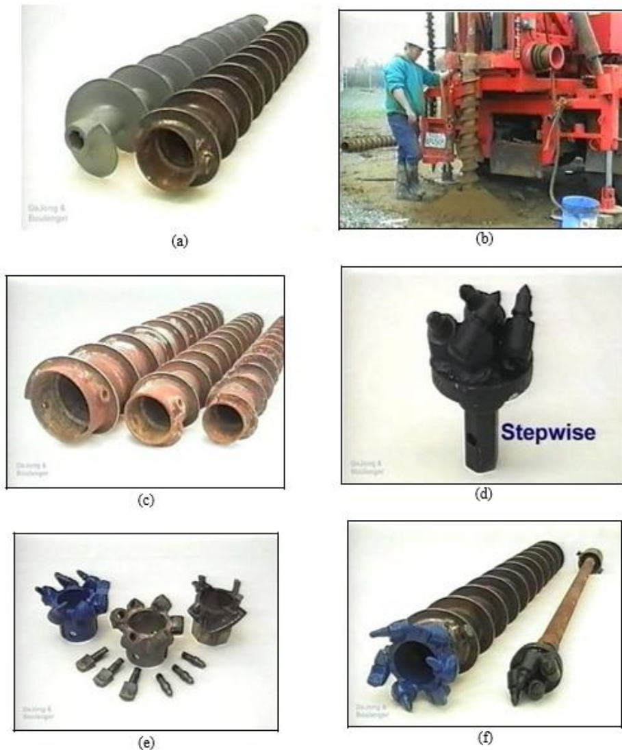
Figure 3-3. Hollow Stem Continuous Flight Auger Drilling Systems: (a) Comparison with solid stem auger; (b) Typical drilling configuration; (c) Sizes of hollow stem auger flights; (d) Stepwise center bit; (e) Outer bits; (f) Outer and inner assembly.
