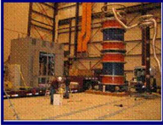
Figure: Testing of Zenergy's FCL device
