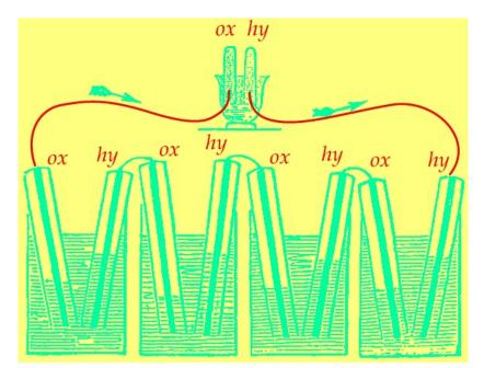
In 1839, William Grove, a British jurist and amateur physicist, first discovered the principle of the fuel cell. Grove utilized four large cells, each containing hydrogen and oxygen, to produce electric power which was then used to split the water in the smaller upper cell into hydrogen and oxygen.
