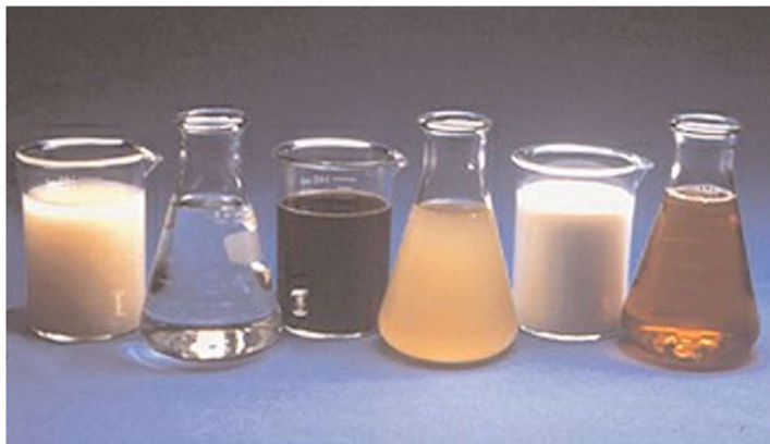
Fig. 1. Liquid admixtures, from left to right: antiwashout admixture, shrinkage reducer, water reducer, foaming agent, corrosion inhibitor, and air-entraining admixture. (69795)
